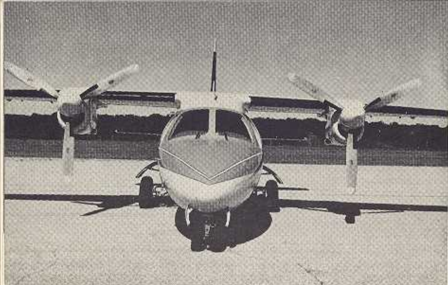
This view of the MOONEY MU-2 gives away some of its secrets: the small low-drag engine nacelles, a very clean fuselage, the low cg, the extra fuselage width, the actual width of the main landing gear.
